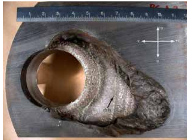
Extensive corrosion of the reactor pressure vessel head of the Davis-Besse nuclear reactor.
