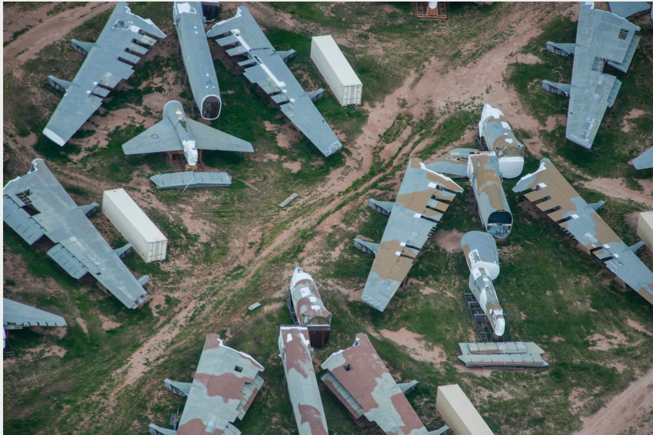
FIGURE 23. AERIAL IMAGE OF DISMANTLED B-52 STRATOFORTRESS BOMBERS EXPOSED TO SATELLITES IN THE EARLY 1990S, IN ACCORDANCE WITH START I PROVISIONS. UNDER NEW START, THE ELIMINATION OF HEAVY BOMBERS INCLUDES CUTTING UP THE FUSELAGE AND EXPOSING IT FOR A PERIOD OF AT LEAST 60 DAYS. IMAGE: JIM GARAMONE, "U.S., RUSSIA EXTEND ARMS REDUCTION TREATY," U.S. DEPARTMENT OF DEFENSE, 4 FEBRUARY 2021, HTTPS://WWW.DEFENSE.GOV/NEWS/NEWS-STORIES/ARTICLE/ARTICLE/2493593/US-RUSSIA-EXTEND-ARMS-REDUC-TION-TREATY/ .
