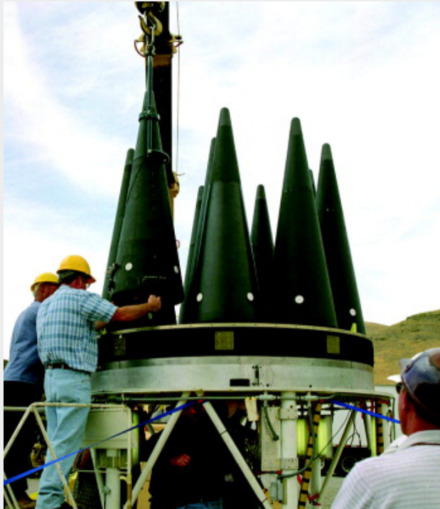
FIGURE 17. BY REMOVING THE MISSILE SHROUD, REENTRY VEHICLES COULD BE EXPOSED TO OVERPASSING SENSORS, ALLOWING FOR COUNTING. THIS IMAGE SHOWS THE FRONT SECTION OF THE PEACEKEEPER MISSILE, WHICH CARRIED 10 RVS WITH W87S WARHEADS. THESE WERE REFURBISHED TO EXTEND THEIR LONG-TERM USE ON MINUTEMAN III ICBMS. SOURCE: LAWRENCE LIVERMORE NATIONAL LABORATORY, "ICBM WARHEADS WITH MODERN SAFETY FEATURES," 1986, HTTPS://WWW.LLNL.GOV/SITES/WWW/FILES/1986.PDF .
