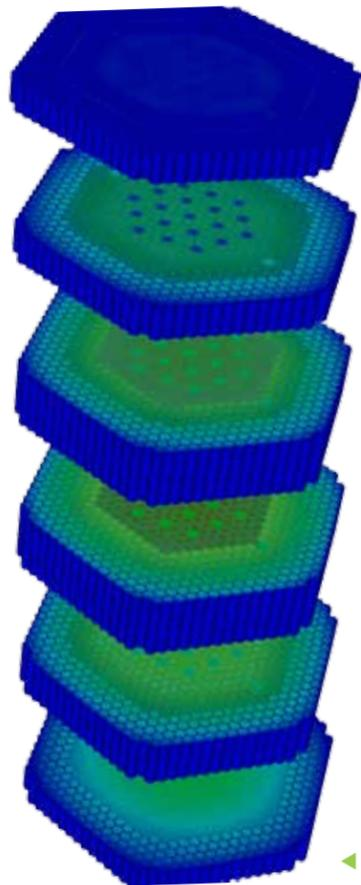
◀ Slices from a full core SN2ND calculation showing the axial power distribution (log scale) in the MONJU reactor.
