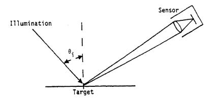
Figure 2. Illumination and Viewing Geometry.
