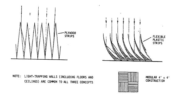
Figure 11. Light-Trapping Wall Designs.
