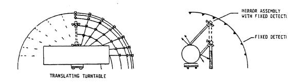
Figure 9. Concept A (Translating and Rotating Object/Movable Optics)
