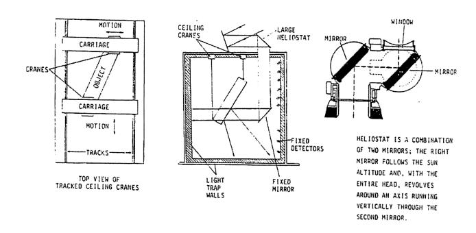
Figure 10. Concept B (Movable Object/Stationary Illumination).
