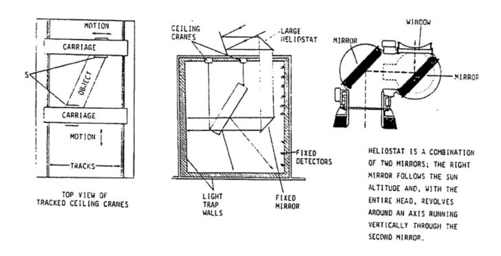
Figure 10. Concept B (Movable Object/Stationary Illumination).
