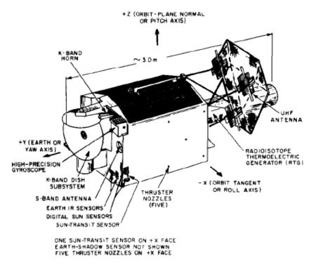
Fig. 1 Lincoln Experimental Satellites (LES) 8 and 9
