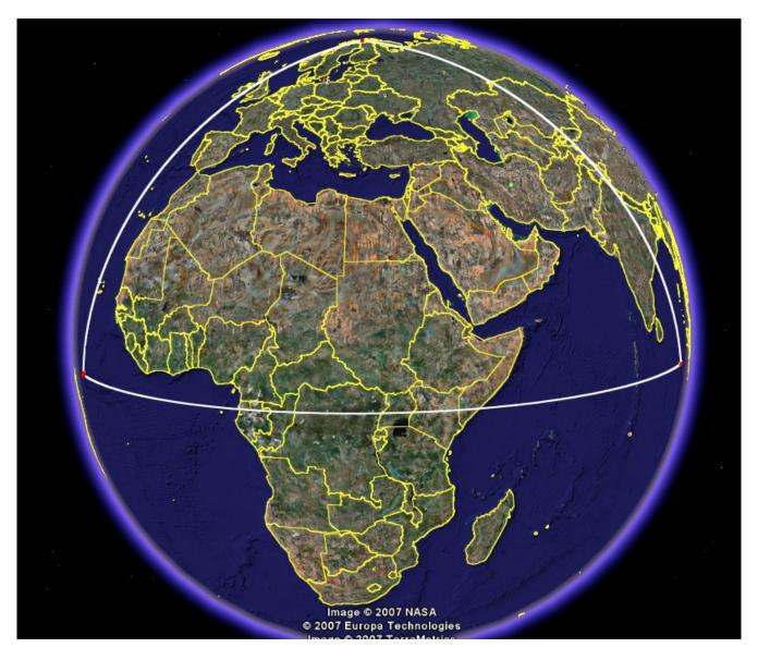
Segment of Geostationary Arc Visible from Vardo, approximately 30 W to 90 E
