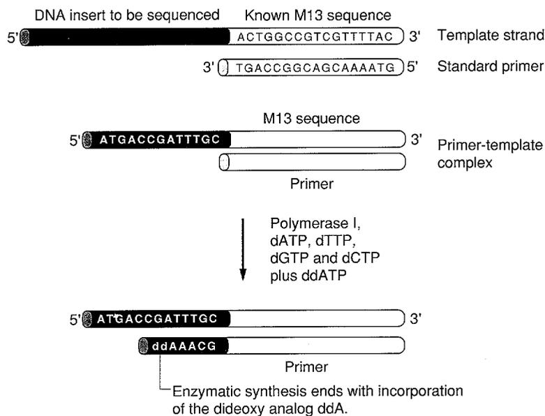
Incorporation of ddATP rather than dATP is random so all possible strands ending at ddATP are synthesized in the reaction.
