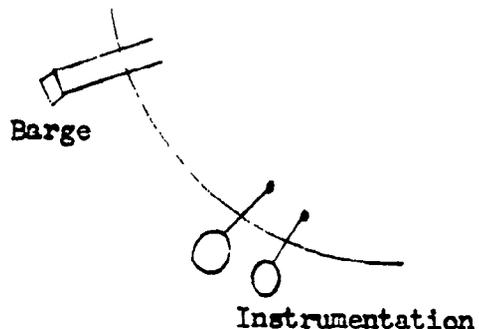
For the lagoon measurements, they would participate in the shot recommended by LMSL as a good one, using a series of stations (probably three, possibly four) which would contain probably six to eight pressure-sensing elements per station, and in addition employing ball crusher gauges for peak pressure.
