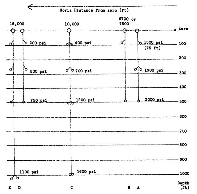
Instrument Line "A" is a 4-channel NOL system; "B", a Hastings system; "C" is an 8-channel Wiancko system.
