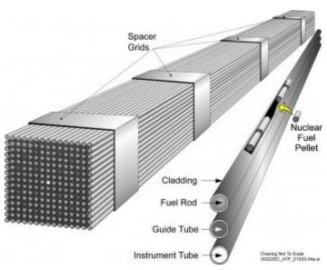
Figure 1. Example of a Nuclear Fuel Assembly
