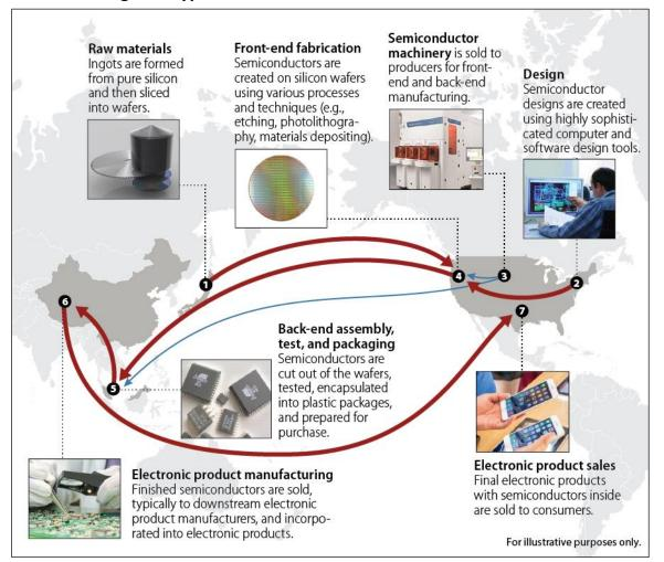
Figure 2. Typical Global Semiconductor Production Pattern
