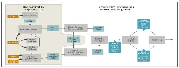
Figure 1. The Iron and Steel Manufacturing Process
