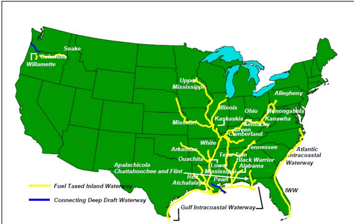
Figure 1. Fuel-Taxed Inland Waterway System
