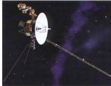
**Figure 10.** Artist's conception of the Voyager 1 spacecraft in its interstellar cruise mode. The three MHW-RTGs are shown mounted on a boom below the spacecraft bus. The high-gain antenna is 3.7-m in diameter. (NASA)
