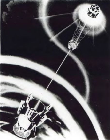
Figure 5. Artist's conception of the Transit 5BN-1 navigational satellite in orbit. The SNAP-9A RTG is mounted at the lower left in this drawing. Transit 5BN-1 was the first spacecraft to be totally powered by a nuclear power source. Transit 5BN-1 was an octagonal prism 45.7-cm across by 30.5-cm high. (JHU/APL)
