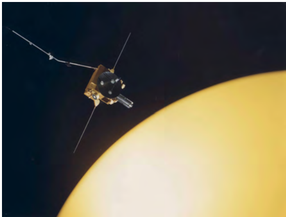
Figure 13. Artist's conception of Ulysses flying over the Sun (the spacecraft does not come this close). The GPHS-RTG is shown mounted on the lower right hand side of the spacecraft. The high-gain antenna is 1.65-m in diameter. (ESA/NASA)
