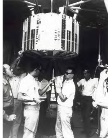
Figure 4. Paul J. Dick preparing to install the SNAP-3B7 RTG on the Transit 4A satellite, June 1961.
