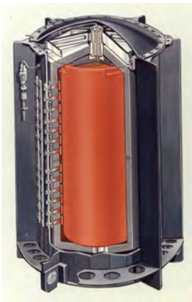
Figure 9. Cutaway of the MHW-RTG which was used on LES 8/9 and Voyager 1/2. The overall diameter was 39.73 cm and the length was 58.31 cm. The average flight mass for Voyager 1/2 was 37.69 kg. (ERDA/GE)
