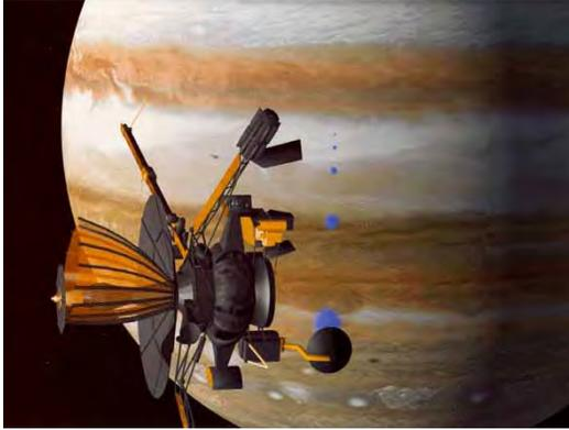
**Figure 12.** Artist's concept of Galileo arriving at Jupiter. One of the GPHS-RTGs is shown at the top mounted on a boom. (NASA)
