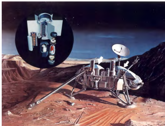
Figure 7. Artist's conception of a Viking Lander on the surface of Mars. A cutaway of the Viking/SNAP-19 RTG is shown as an insert with arrows indicating where the two SNAP-19 RTGs were placed on the Lander. The overall RTG diameter (across fins) was 58.7 cm and the overall length was 40.4 cm. The mass was 15.2 kg. (NASA/ERDA/Teledyne)
