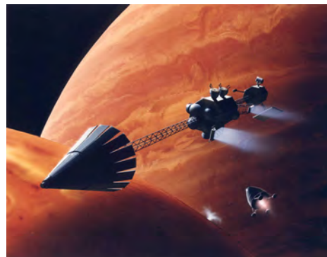
Figure 17. Artist's conception of an SP-100-powered Jovian grand tour mission using ion thrusters. (NASA)
