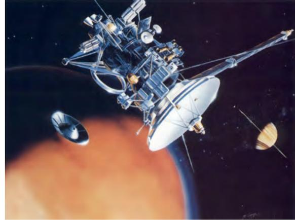
**Figure 14.** Artist's conception of the Huygens probe being released from the Cassini spacecraft over Titan, the largest satellite of Saturn. Two of the three GPHS-RTGs can be seen mounted to Cassini in the upper left in the figure. The high-gain antenna is 4-m in diameter. (NASA)
