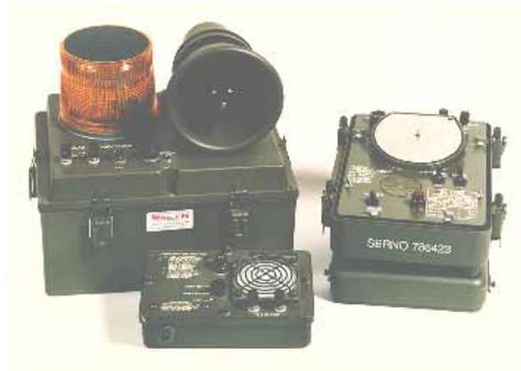
**5.1.1. Purpose.** The ALAD provides the user with an automatic liquid chemical agent detector. ALADs are intended for use with existing vapor detectors.
