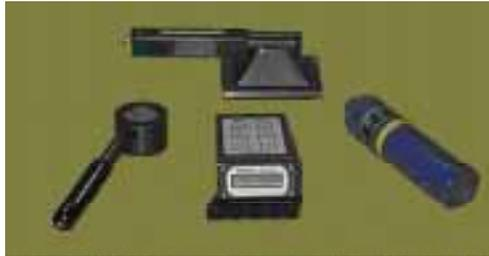
**5.9.1. Purpose.** The ADM-300 RADIAC meter will locate and measure low and high intensity gamma rays or detect beta particles. When used with external probes, it will locate and measure alpha, gamma, x-ray and neutron radiation, and detect the presence of beta.
