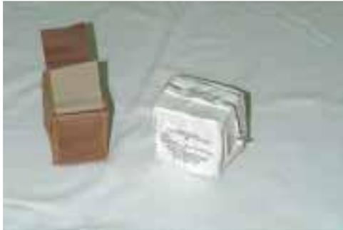
**3.2.1. Purpose.** The M9 paper will detect G and V Nerve agents and H and L blister agents. M9 paper manually provides a visual image of liquid chemical agent droplets. When worn on protective clothing or attached to equipment, M9 paper provides one rapid assessment of detection.
