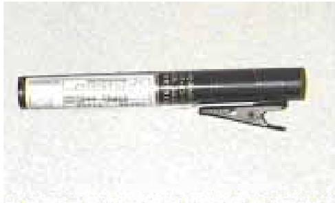
**5.8.1. Purpose.** The dosimeter detects and measures cumulative exposure to X-ray and gamma-ray radiation. The dosimeter can be used for individual or area measurement for total radiation exposure. This survey meter is designed for large area surveying to find the extent and intensity of radioactive contamination. It can also be used for area and personnel monitoring to determine the presence and intensity of residual radiation.
