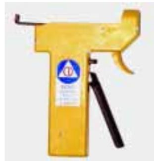
**5.7.1. Purpose.** The charger provides the user with a portable unit designed to provide the necessary voltage to charge, illuminate, and read the IM-143 dosimeter.
