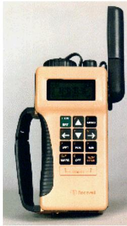
**6.4.1. Purpose.** The Global Positioning System (GPS) provides the user with global positioning and siting capabilities. The AN/PSN-11 will provide data for missions such as general navigation, siting/surveying, tactical reconnaissance, close air support, engineer surveying, electronic warfare (EW) operations, and ground-based forward air control.
