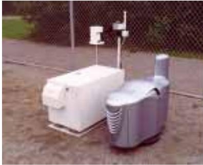
**5.6.1. Purpose.** Portal Shield provides the user with a biological detection system with a chemical add-on consisting of the ACADA. The system is hard-wired with comm back up to provide continuous information through a computer terminal located at the command and control centers chosen by the installation. The computer terminal indicates when an agent is detected and can identify the specific biological agent triggered upon in near real time.
