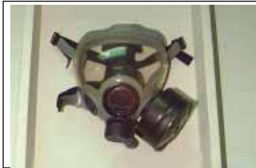
**2.3.1. Purpose.** The MCU-2A/P mask with a serviceable canister filter installed protects the faces, eyes, and respiratory tract from chemical and biological warfare agents and radioactive dust particles. A properly worn mask provides a gas-tight face seal which prevents unfiltered air from reaching the wearer's respiratory system.
