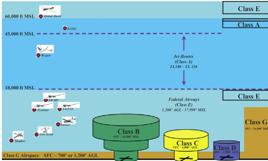
Figure 3. FAA Airspace Classification & Relative UAS Operating Areas
