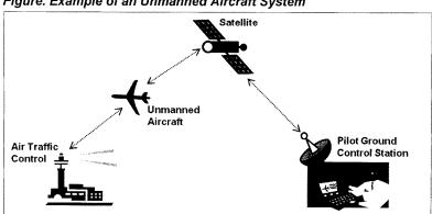
Figure. Example of an Unmanned Aircraft System
