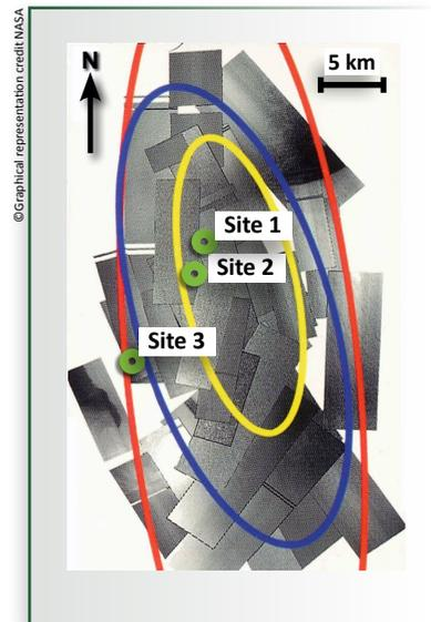
**Figure 7. Site Locations Compared to Predicted MPL Landing Site Ellipses<sup>3</sup>**
