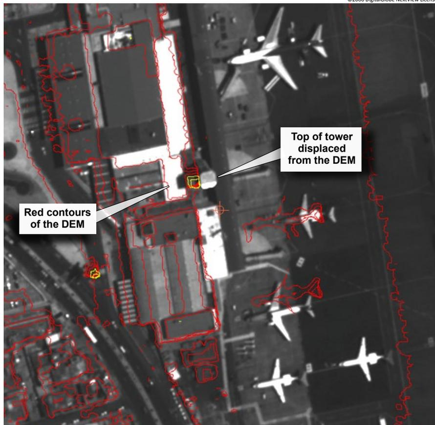
Figure 8. Misregistered Image and LIDAR DEM
