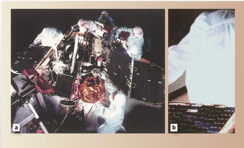
Figure 16. a) MPL During Assembly and Testing, b) Closeup of Garment Reflection in an MPL Solar Panel<sup>3</sup>
