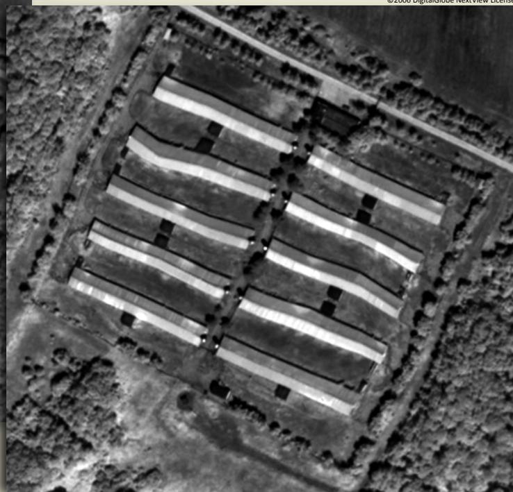
Figure 10. The Same Buildings After Orthorectification With a Bad DEM
