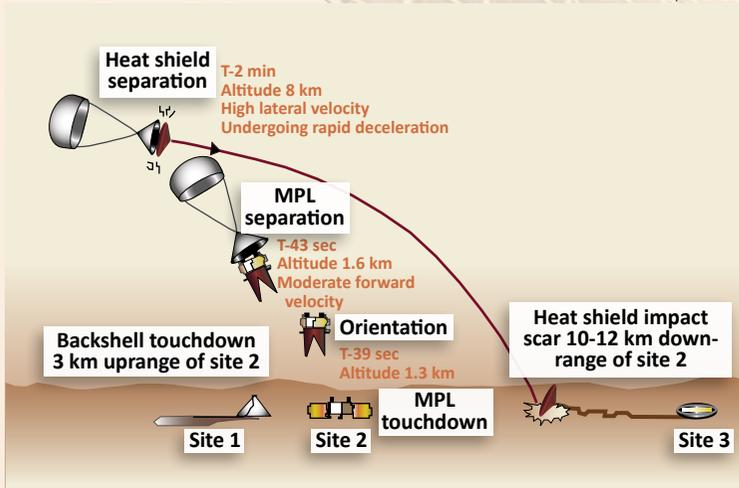
Figure 28. Postulated MPL EDL Scenario Based on Search Findings (Side View)<sup>3</sup>
