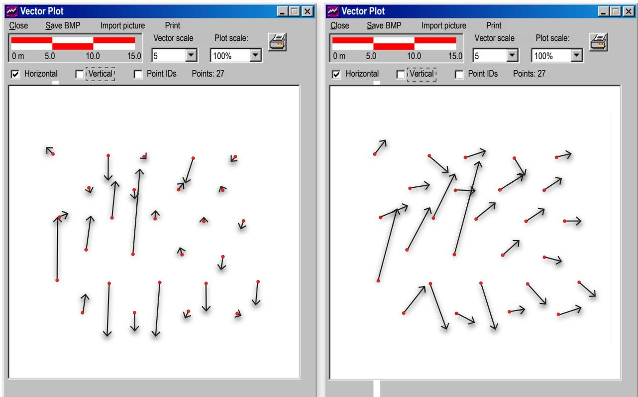
Figure 6. Look Angle-DEM Interaction Errors (left) and Total Errors (right)
