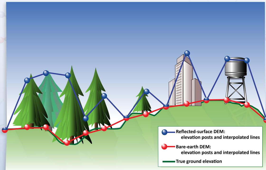
Figure 3. Differences Between Two Types of DEMs and True Ground Elevation (Cross Section)
