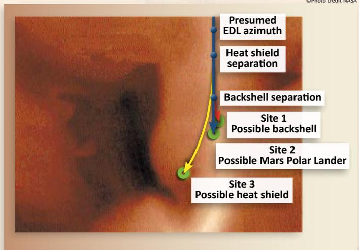
Figure 29. Postulated MPL EDL Scenario Based on Search Findings (Top View)<sup>3</sup>
