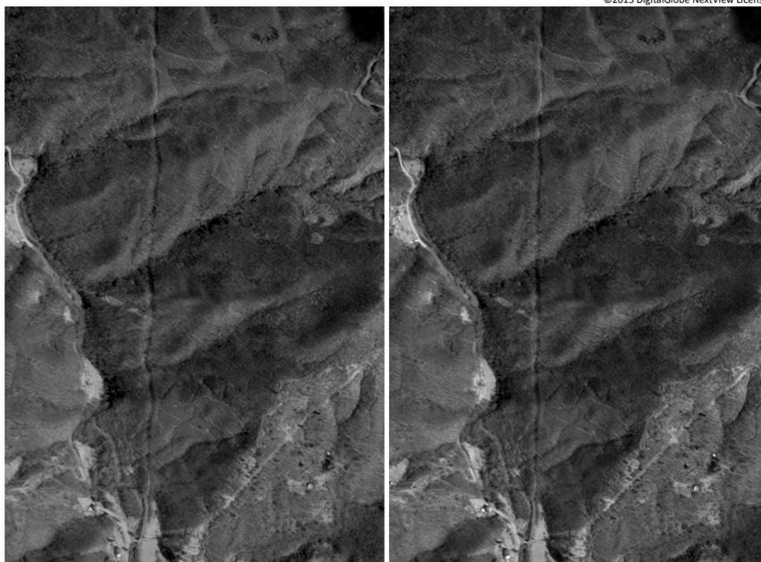
**Figure 1. Terrain Effects Wiggle the Path of a Powerline (left); Orthorectification Straightens the Path (right)**
