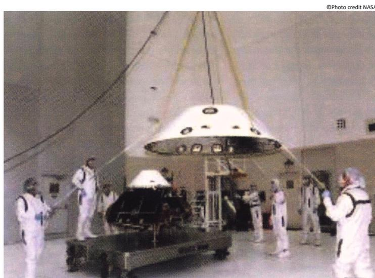
Figure 21. MPL Backshell During Payload Integration<sup>3</sup>
