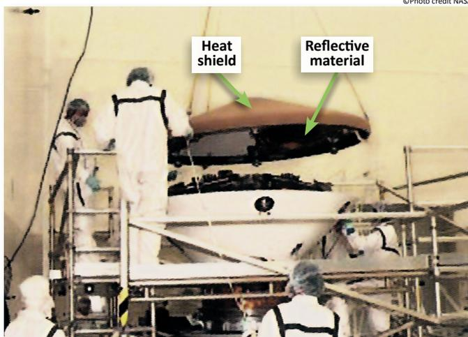
Figure 27. MPL Heat Shield During Payload Integration
