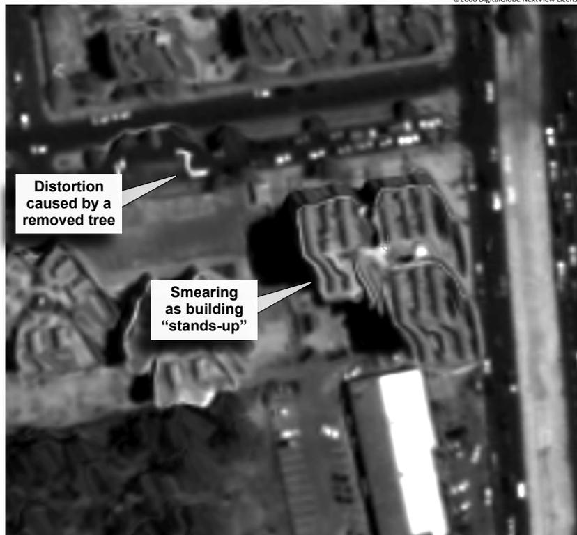
Figure 7. Problems With a High-Resolution LIDAR DEM
