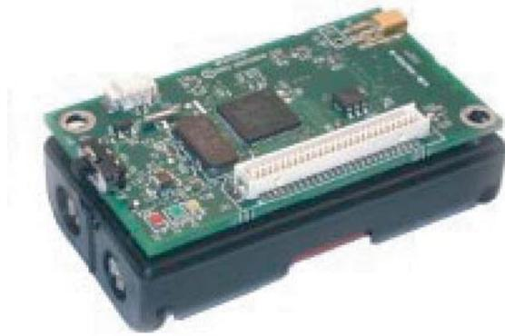
Figure 20: The Crossbow MICA2 wireless node
