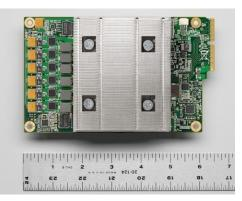
Figure 25. A photo of Google's tensor processing unit (TPU). Few details of this chip have been released. All that is known is that it gives  $10 \times$  the efficiency as some undisclosed alternative on inference.
