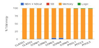
Figure 23. Because it fetches all data from external DRAM. the power dissipation of DianNao is completely dominated by memory fetch.
