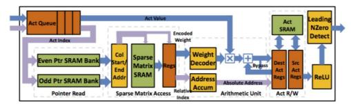
Figure 24. Block diagram of the efficient inference engine (EIE). EIE keeps the weights in a highly-compressed form (compressed  $240\times$ ) by pruning the network and coding the non-zero weights using trained quantization. The special-purpose hardware is tailored to operate efficiently on this sparse, encoded representation.
