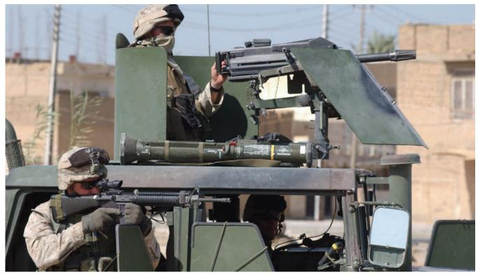
Photo by Cpl Matthew S. Richards The Humvees of BLT 1/4 carried a wide assortment of weapons, including TOW missiles, AT-4 rocket launchers, .50-caliber machine guns, 7.62mm M240G machine guns, and MK19 automatic grenade launchers.
