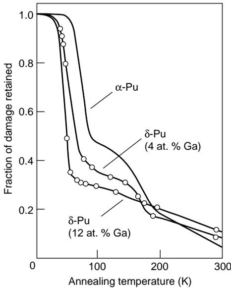
**Figure 2. Recovery of Self-Irradiation Damage**
