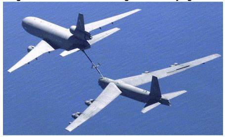
Figure 1. USAF KC-10 Refueling B-52 with Flying Boom
