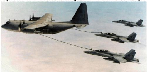
Figure 2. USMC KC-130 Refueling F/A-18s with Hose-and-Drogue
