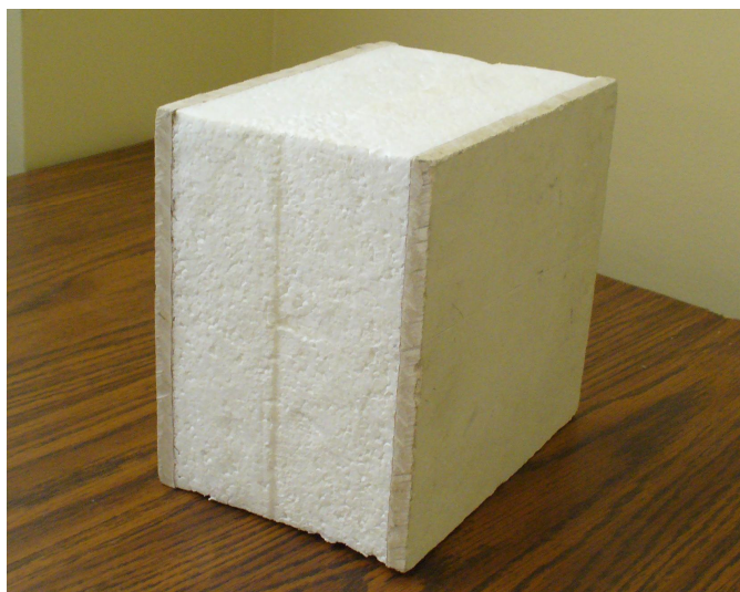
Figure 1 – Structural Insulated Panel with Cement Fiber Facing
