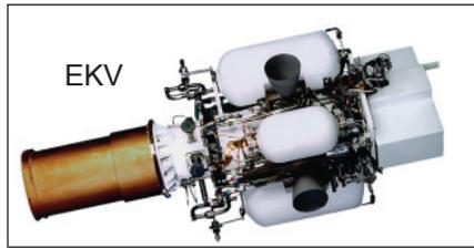
The ground-based interceptors are comprised of a booster vehicle and an exoatmospheric kill vehicle (EKV). Upon launch, the booster flies to a projected intercept point and releases the EKV which then uses on-board sensors (with assistance from ground-based assets) to acquire the target ballistic missile. The EKV performs final discrimination and steers itself to collide with the enemy warhead, destroying it by the sheer kinetic force of impact.
