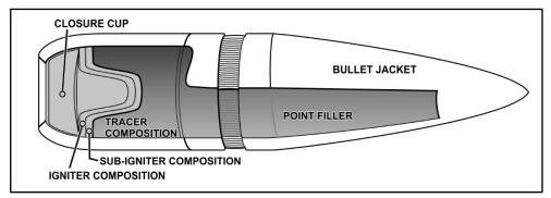
Figure A-7. Ball with tracer cartridge
