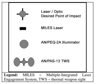
Figure G-1. 10-meter target offset symbols
