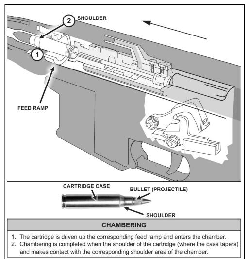
Figure 2-4. Chambering example
