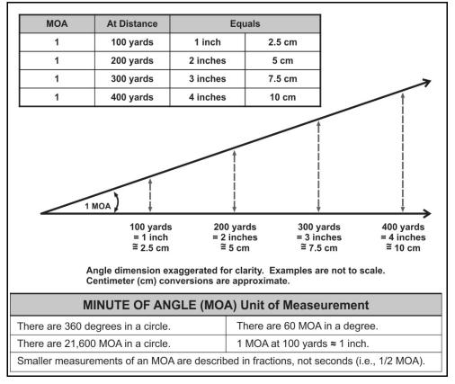
Figure 3-1. Minute of angle example
