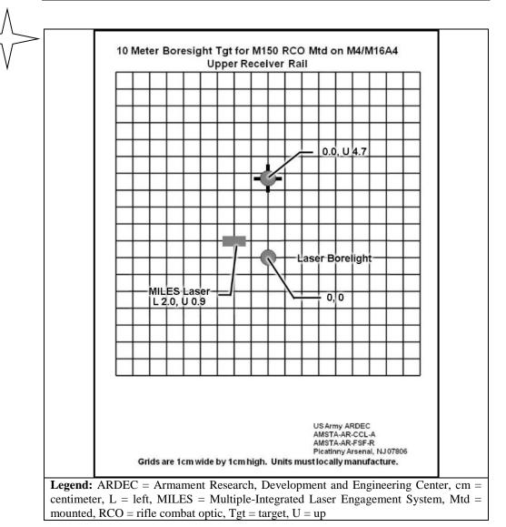
Figure G-4. 300-meter zero of the advanced combat optical gunsight
