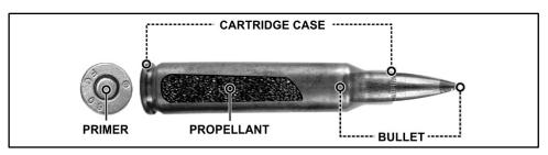
Figure A-1. Small arms ammunition cartridges
