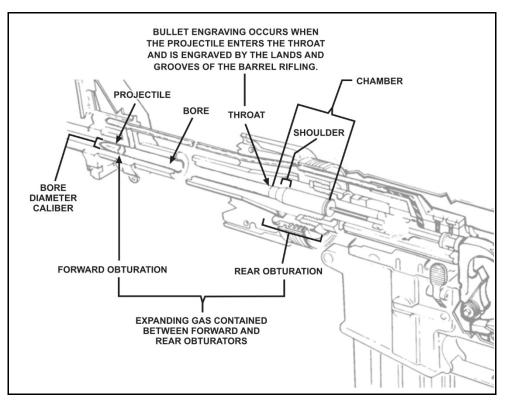
Figure B-1. Internal ballistic terms
