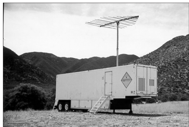
The Vulnerability Mobile Transmitter-A provides programmable signal jamming capability in the 2 MHz to 1,000 MHz range.
