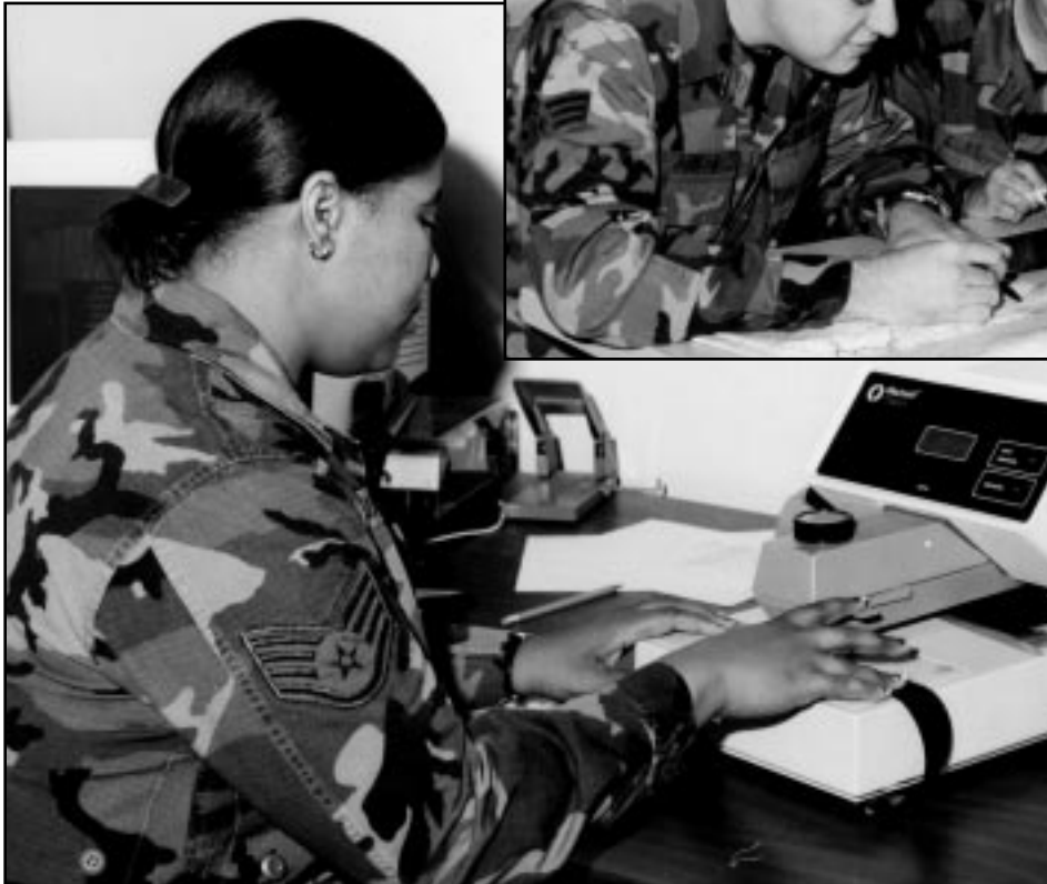
Upper right, Staff Sgt. Stacey Spears helps fellow imagery analyst Senior Airman Greg Johnson plot coordinates on a map. Lower left, Staff Sgt. Shawna Brown, visual information photography specialist, measures the black and white contrast of film by using a densitometer.
