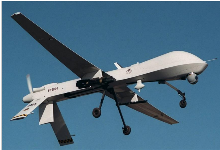
Figure 2. Air Force MQ-1 Predator Armed with a Hellfire Missile
