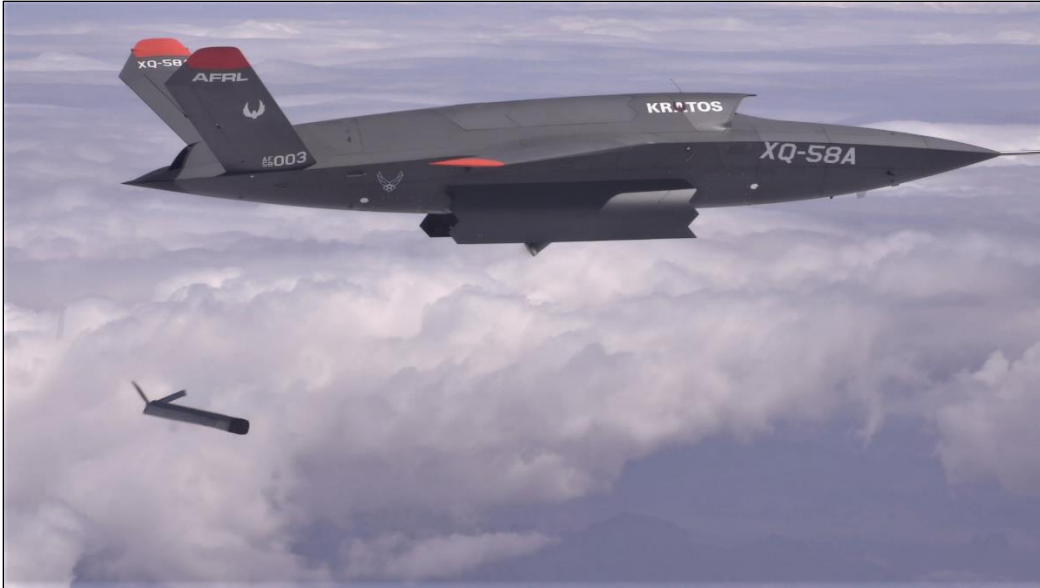
Figure 6. Valkyrie UAS Deploys ALTIUS-600 Small UAS
