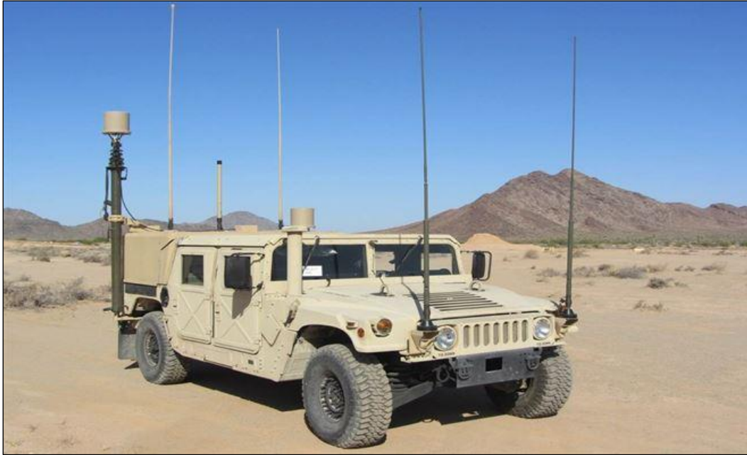
Figure 9. High Mobility Multipurpose Wheeled Vehicle Equipped with CESAS II
