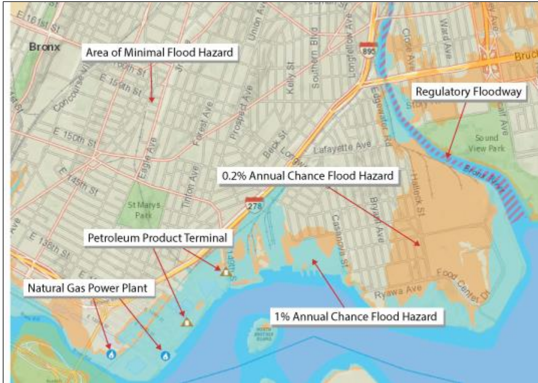
Figure B-2. Example Flood Vulnerability Assessment Map
