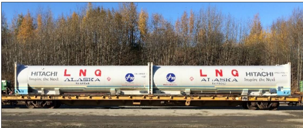
Figure 1. Alaska LNG Shipment on Flatbed Rail Cars in ISO Containers
