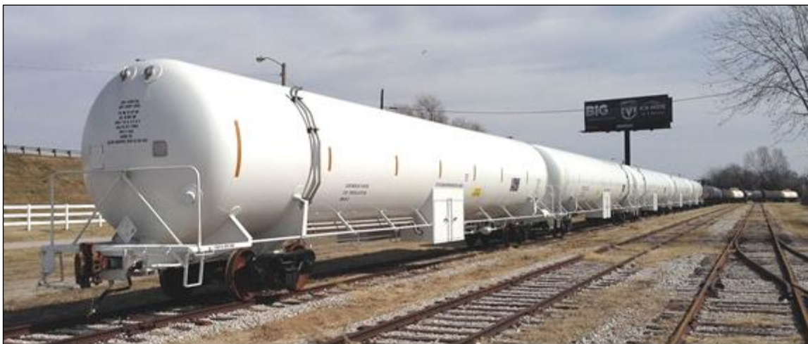
Figure 2. Insulated Rail Tank Cars Proposed for LNG
