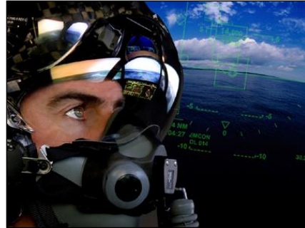
Figure 2. F-35 Helmet Mounted Display
