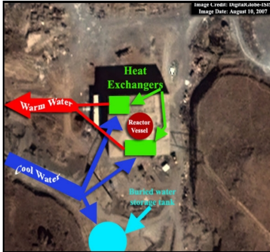
Figure 33. DigitalGlobe satellite imagery from August 10, 2007 of the reactor building. Cool water is pumped from the river and into a buried water storage tank and the reactor building's heat exchangers. The heat exchangers transfer the heat from the gas to the water from the river. The warm water is then discharged and piped back over to the river.
