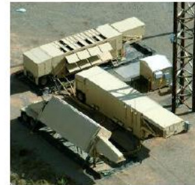
The FBX-T radar is designed to acquire and track targets early in the trajectory.
