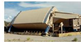
The FBX-T radar is designed to acquire and track targets early in the trajectory.
