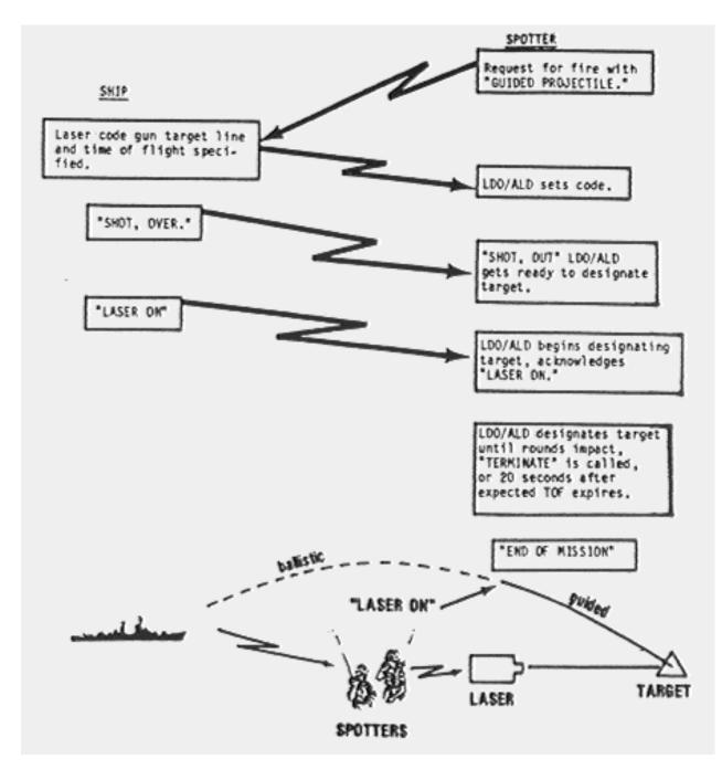
Figure B-3. Ground and Airborne Laser Designation Procedures for NGFS Call for Fire Mission
