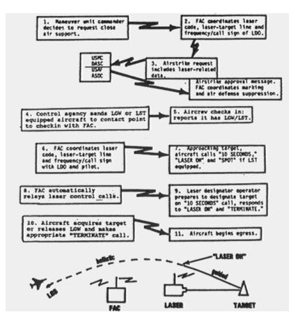
Figure B-4. Procedures for Aircraft with LST/LGW
