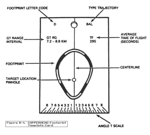
Figure B-1. COPPERHEAD Footprint Template Card
