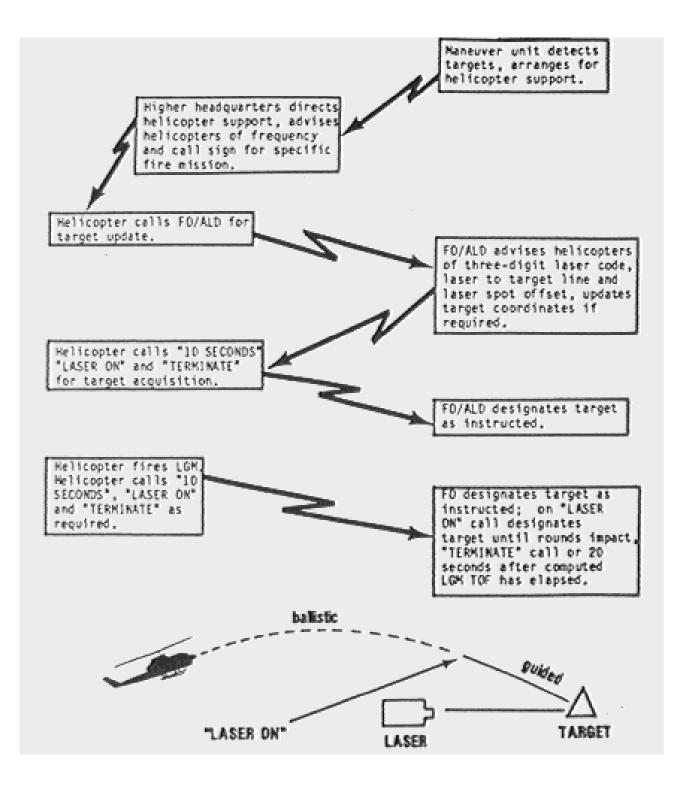
Figure B-8. Procedures for Helicopters with LST/LGM
