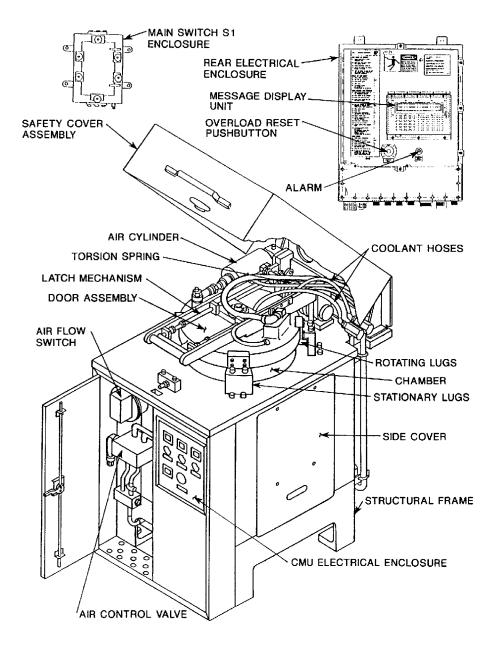
Figure 593-2-3 Compress Melt Unit
