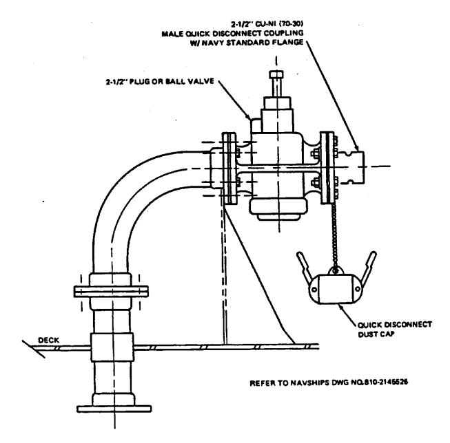
Figure 593-3-3 Surface Ship Oily Waste Discharge Connection
