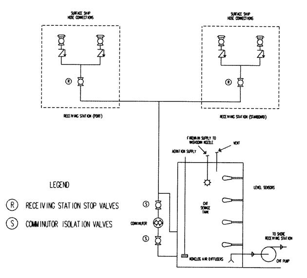
Figure 593-4-5 Surface Ship Tender Receiving Station
