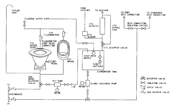
Figure 593-4-7 GATX MK I Evaporative Toilet System
