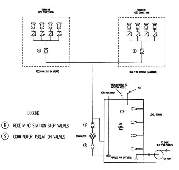
Figure 593-4-6 Submarine Tender Receiving Station
