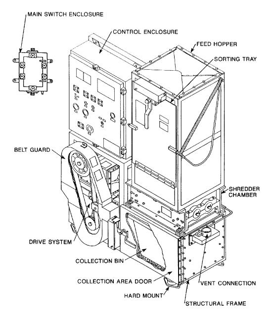
Figure 593-2-6 Metal / Glass Shredder
