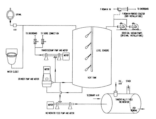
Figure 593-4-8 JERED Vacuum Collection and Incineration System
