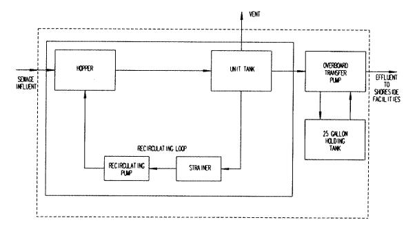
Figure 593-4-10 Koehler-Dayton Marine Sanitation Device Functional Schematic
