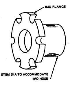
TO ENABLE PIPES OF RECEPTION FACILITIES TO BE CONNECTED WITH THE SHIP'S DISCHARGE PIPE LINES FOR THE RESIDUES FROM MACHINERY BILGES, LINES SHALL BE FITTED WITH A STANDARD DISCHARGE CONNECTION IN ACCORDANCE WITH THE FOLLOWING TABLE:
