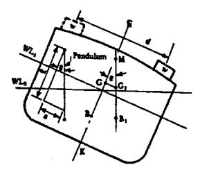
Figure 096-2-1. Effect of Weight(s) on Angle of List
