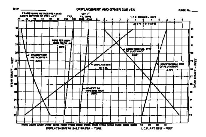
Figure 096-2-2. Sample Sheet for Plotting Displacement and Other Curves
