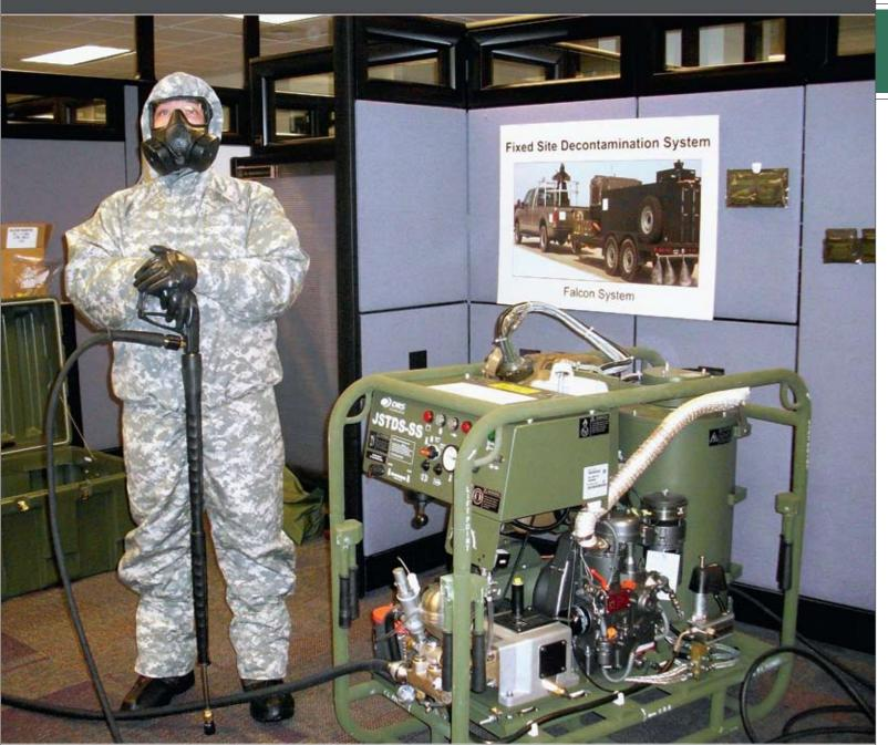
Joint Service Transportable Decontamination System (JSTDS) – Small Scale (SS)
