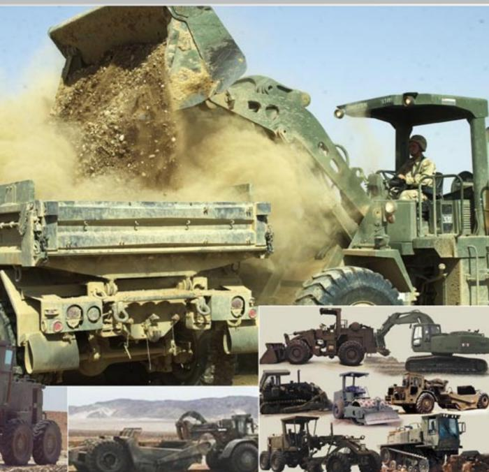
The Construction Equipment Service Life Extension Program (CE SLEP) returns vehicles to a like-new condition that meets their original purchase description. The CE SLEP extends the life of the vehicle 10 to 15 years. Some of the vehicles currently being refurbished are dozers, scrapers, graders, loaders, and water distributors.
